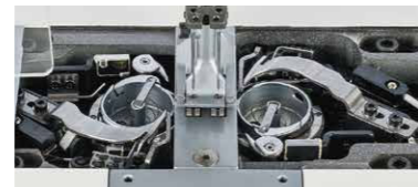
B: Bed slide with an open / close sensor
