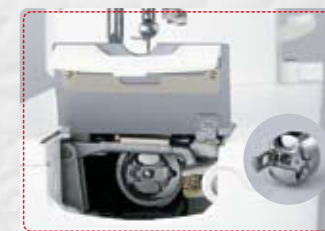
● Horizontal-axis Full-rotary Hook Create perfectly balanced stitches for beautiful seams. Bobbin thread tension is also adjustable.
