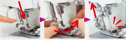
Step.1 Lower the threading lever.
