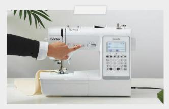
Press the thread cutter button to snip your threads at the end of sewing. (A150 model only)
