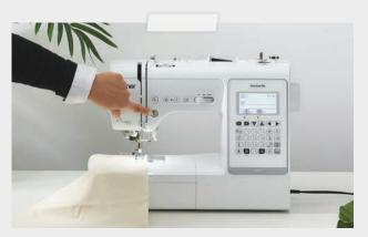
Press the Start/Stop button to use the machine without the foot controller.
